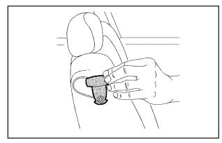
Remove the guide from the storage clip on the side of the rear seatback.
